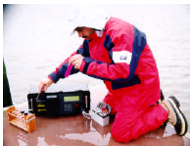
The Model 10-AU Field Fluorometer in use in a fluorescent tracer study.
