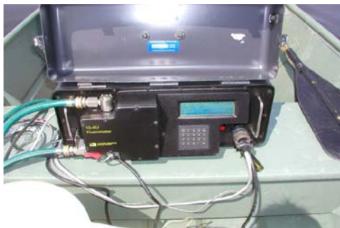
Figure 2: The Turner Designs 10-AU Fluorometer set up for flow through sampling of Brighteners (Hagedorn et al 2002).
