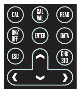
**CAL** – Is used to calibrate the instrument. See section 2.3 for instructions and procedure on how to calibrate the *Aqua*Flash.
