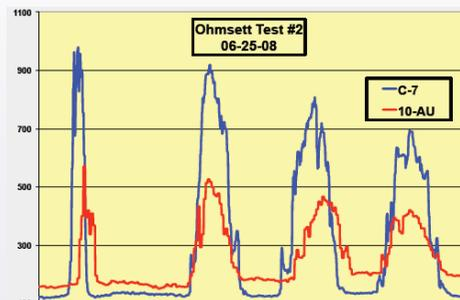
Oil spill response tank test in Leonardo, NJ comparing 10-AU fluorometer with C3 optics used for detecting dispersed oil.
